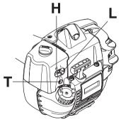
The L and H-jets are used to adjust the supply of fuel
